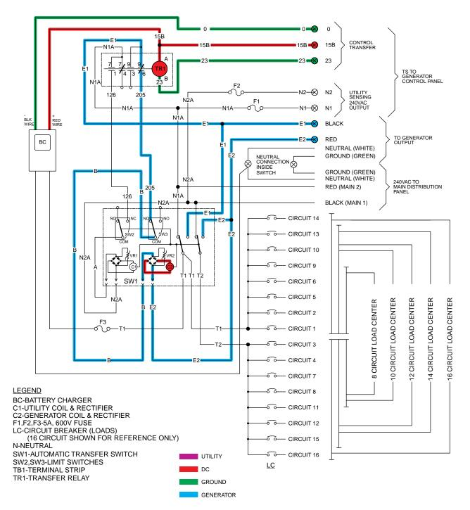
Figure 5. Transfer Action to Standby Position
